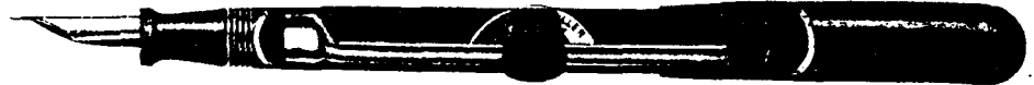
Sectional View No. 2, showing "Crescent-Filler" released, and the Elastic Ink Reservoir compressed ready for filling.
